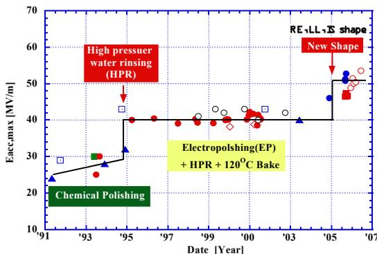
Figure 4: The breakthrough in high gradient of 50MV/m.
