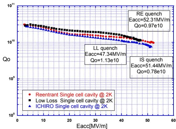
Figure 3: The results of high gradient measurements.
