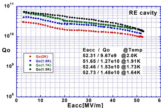
Figure 6: Temperature dependence of gradient.
