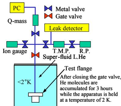
Figure 4: Experimental set up for the super-fluid He leak rate measurement using a pressure build-up method.
