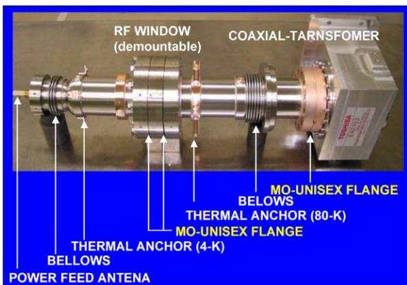
Figure 8: De-mountable type input power coupler using the MO type unisex flange. An input coupler consists of four parts, a coaxial waveguide transformer, a coaxial waveguide on the warm side, an rf window and a coaxial waveguide on the cold side.
