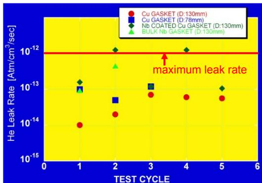
Figure 7: He leak rate using the pressure build up method at super-fluid He temperatures (below 2-°K) for various gasket materials.
