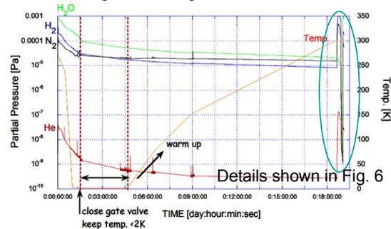
Figure 5: Q-mass measurements of the partial vacuum pressure as a function of time for He, H<sub>2</sub>O, H<sub>2</sub> and N<sub>2</sub> in the over all vacuum system.
