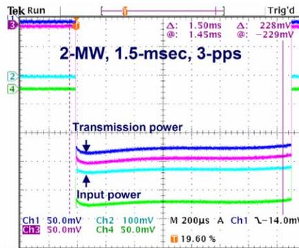
Figure 9: A typical rf waveforms at 2-MW of peak power, 1.5-msec of pulse width and 3-pps of repetition rate.
