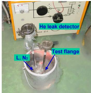
Figure 3: Thermal shock test at liquid N<sub>2</sub> temperature.
