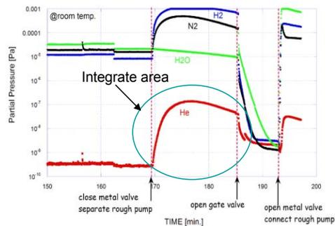
Figure 6: Q-mass measurements for the build up area of the He, H<sub>2</sub>O, N<sub>2</sub> and H<sub>2</sub> in the flange test volume. The area is integrated for 3 hours while the vacuum pump system is isolated by the gate valve.
