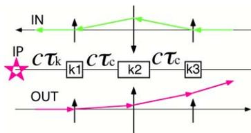
Fig. 7 Three kicker configuration. Bending angles for the incoming bunch (top figure) is exaggerated for clarity.
