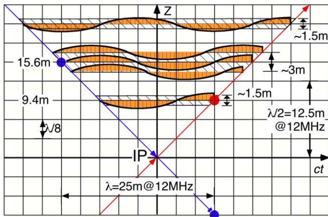
Fig. 8 RF kicker timing chart. The horizontal axis and the vertical axis show time and longitudinal coordinates, respectively. Blue dot shows the bunches going into interaction point (IP), while red one shows leaving bunch. Because both bunches meet at IP, it seems that a bunch coming from the top left corner is reflected at the IP and goes up to the right, which may ease the understanding of this chart.
