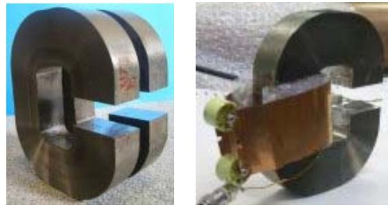
Fig. 5 Large gapped FINEMET core with coupling loop and capacitors for a rough measurement.
