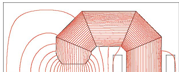
Fig. 6 Magnetic flux distribution in a core. The core material is simulated as anisotropic. Flux concentration at the inner corner and the eddy current loss at the edges of gap may cause problems.
