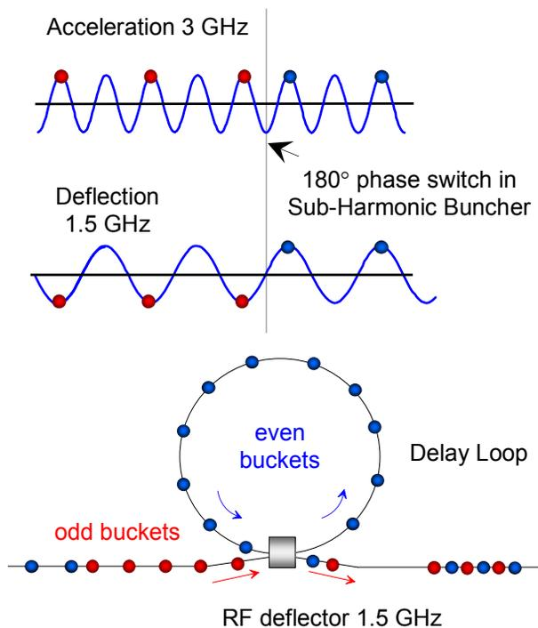
Figure 2: Schematic of the delay loop recombination.
