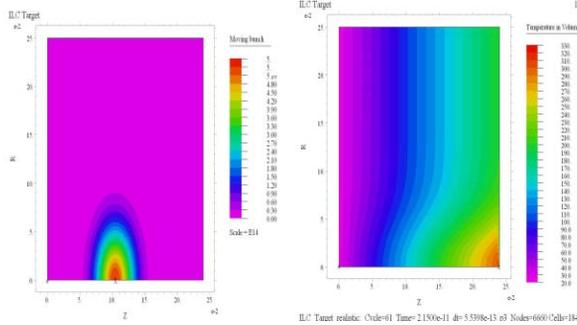
Figure 1: Instant position of the bunch moving in the target, at the left. Isotherms right after the bunch passage, at the right.
