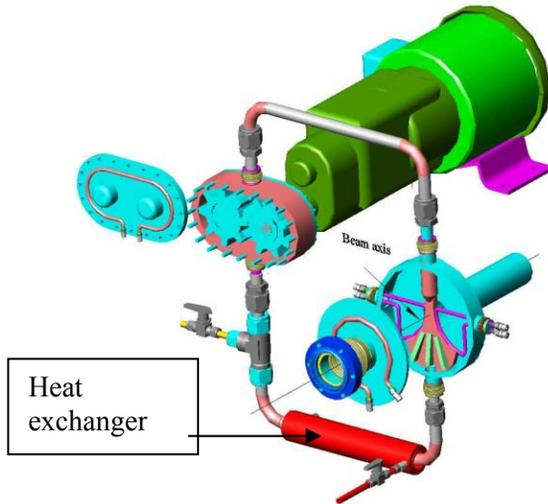
Figure 2: Scheme of liquid target. Diameter of the chamber is  $\sim 10$  cm.
