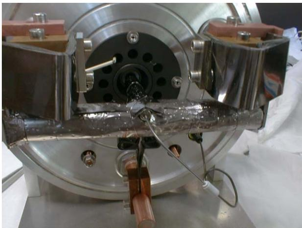
Figure 7: The target ion source system
