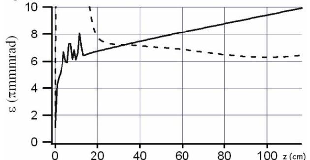
Figure 3 : rms normalised emittance as a function of the distance; PARMELA simulation with the same parameters used in Table 1, without coils (plain line) and with coils (dashed line).
