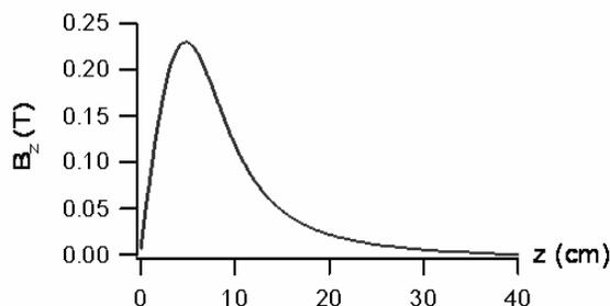
Figure 5 : longitudinal magnetic field simulated with POISSON.
