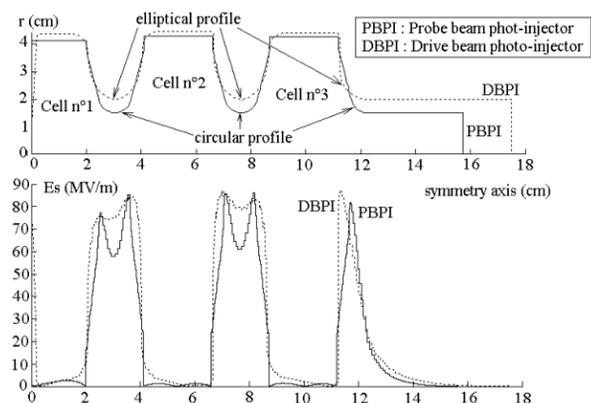
Figure 1 : upper part : 2D profile of PBPI and the DBPI. Lower part: surface electrical field amplitude (for an on-axis maximum field of 80 MV/m).
