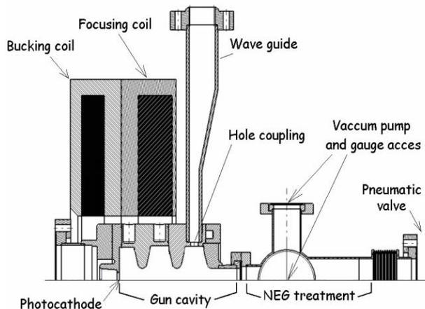
Figure 4 : Sketch of the photo-injector.
