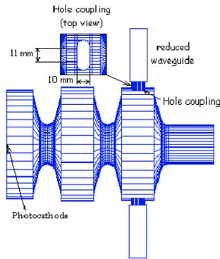
Figure 2 : Sketch of the PBPI with power coupling devices.
