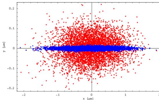
Figure 1 Beam-sizes before (red) and after tuning (blue), from a 1mrad rotation around the s-axis of QD0.
