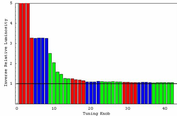
Figure 2 Inverse relative luminosity vs. tuning knob. 1<sup>st</sup> order correction (Red), coupling (Blue), 2<sup>nd</sup> order (Green).
