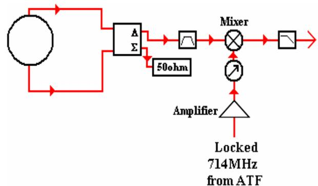
Figure 5: Schematic of BPM signal processor.
