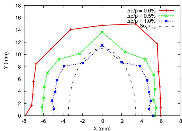
Figure 2: CesrTF dynamic aperture for 0.5% and 1% energy offsets. The dashed curve corresponds to  $3\sigma$  of the the rms size of the injected beam.
