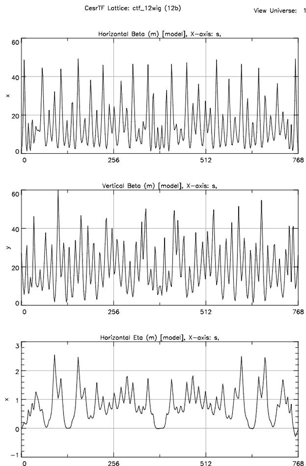
Figure 1: CesrTF Lattice Parameters for 2.0 GeV Operation
