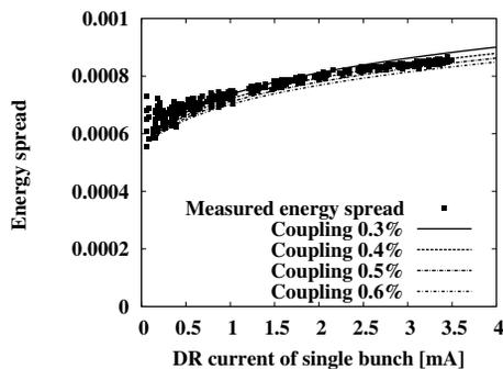
Figure 9: The comparison between the measured momentum spread and calculation
