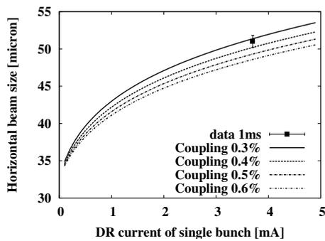
Figure 7: The comparison between the measured horizontal beam size and calculation
