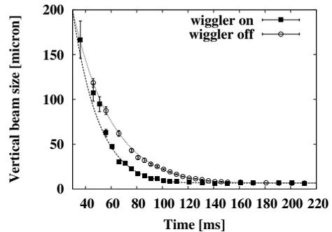
Figure 10: The results of the measured vertical damping time.
