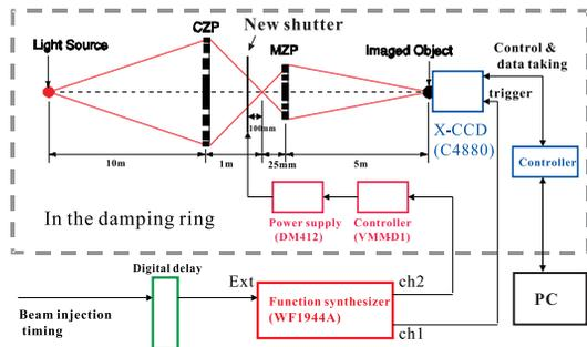
Figure 2: The block diagram of FZP monitor
