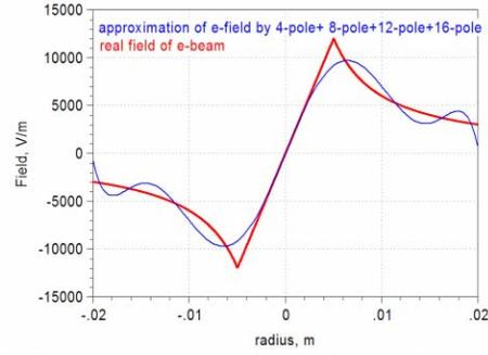
Figure 1: The space charge field of the e-beam with the uniform distribution and its approximation by multipoles.
