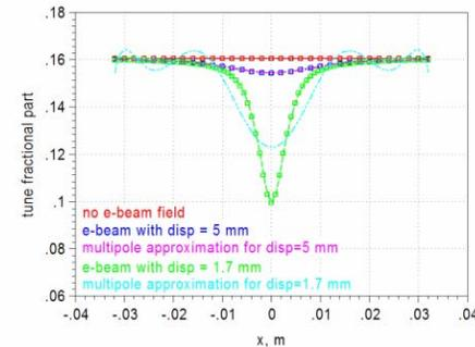
Figure 4: The tune fractional part of anti-proton beam at Gaussian e-beam distribution with  $I_e=1$  A and  $\sigma_e=5$  mm.
