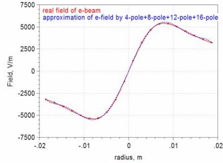
Figure 2: The space charge field of the e-beam with the Gaussian distribution and its approximation by multipoles.
