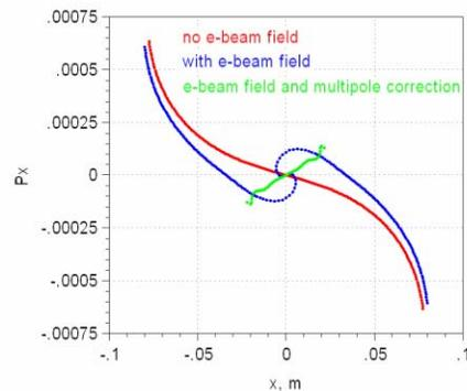
Figure 5: The phase line modification of antiproton beam at the Gaussian electron beam distribution with  $I_e=1$  A and  $\sigma_e=5$  mm.
