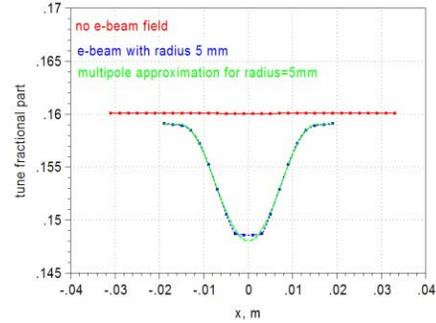
Figure 3: The tune fractional part of anti-proton beam at the uniform e-beam distribution with  $I_e=1$  A and  $r_e=5$  mm.
