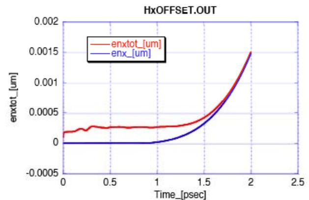
Figure 4: Normalized emittance vs. time for the 1 ps laser, 1 pC case. Blue line: space charge induced emittance Red line: total emittance including laser induced emittance.
