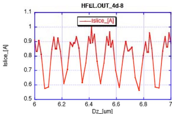
Figure 6: Normalised beam current modulation at the end of the photo-emission process, blow up of Fig. 5. Notice the deep current modulation (40%) on the laser wavelength scale.
