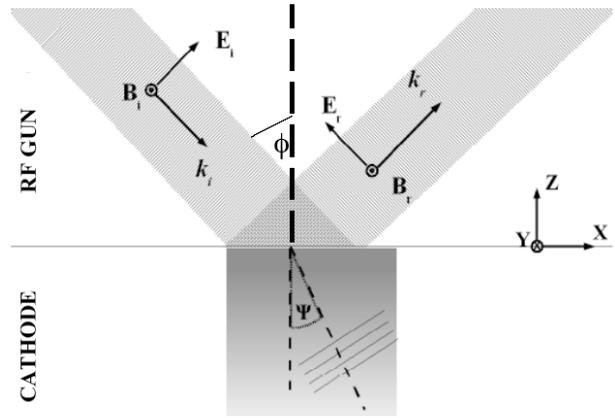
Figure 1: P-polarized plane wave incident on a lossy medium [3].
