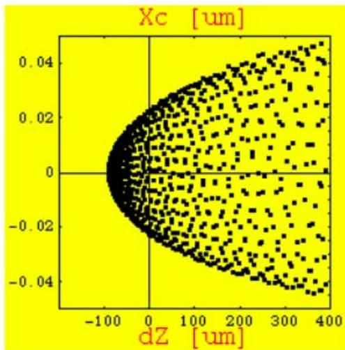
Figure 2: Slice centroids evolution during the interaction with the laser beam. Each dot represents a slice centroid located at a distance dz from the bunch central slice.
