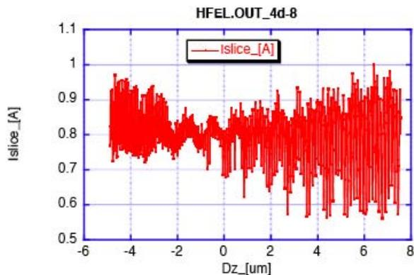
Figure 5: Normalised beam current modulation at the end of the photo-emission process.
