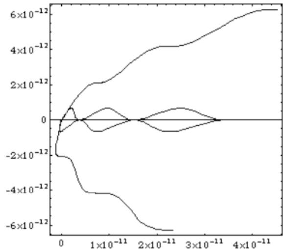
Figure 3: Electron trajectories for different injection phases in a laser field with grazing incidence. (Transverse displacement [m] versus time [s]).
