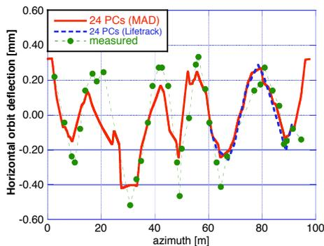
Figure 1: computed orbit deflection due to 24 BBLR interactions for the positron bunch colliding against 10 mA electron bunches.
