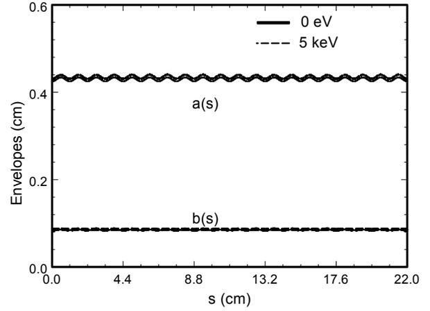
Figure 2: Plots of (a) envelopes  $a(s)$  and  $b(s)$  versus the axial distance  $s$  for the relativistic twisted elliptic beam.
