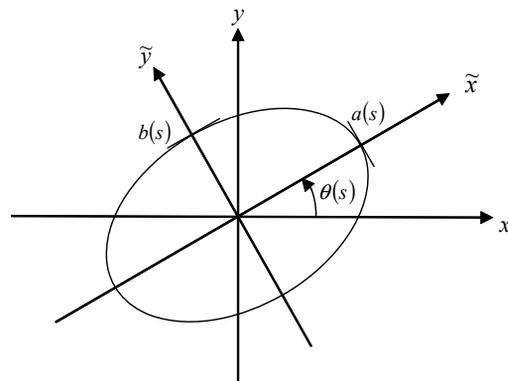
Figure 1: Laboratory and twisted coordinate systems.
