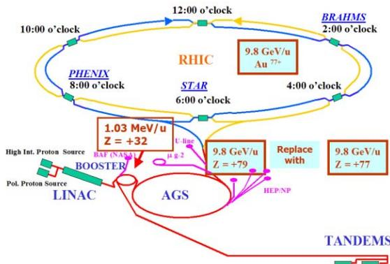
Figure 1: RHIC layout and proposed changes.
