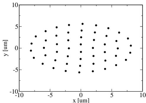
Figure 4: A multi-shell crystalline beam formed with the lattice in Fig. 3 with  $\gamma = 1.45$  and density  $2.1 \times 10^7/m$ .
