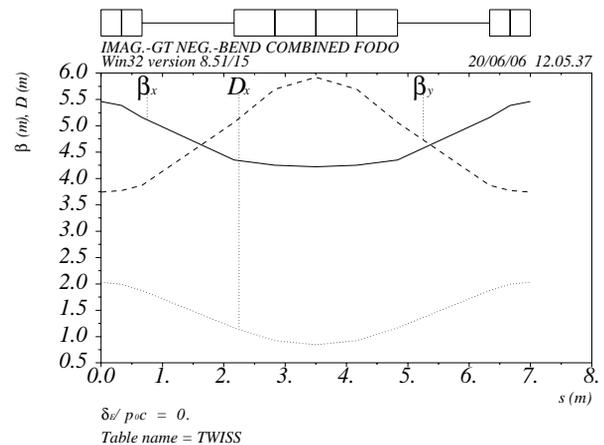
Figure 3: Imaginary- $\gamma_T$  negative-bend lattice with  $87^\circ$  horizontal phase advance. The middle (positive) bend is of combined-function (dipole and defocusing quadrupole).
