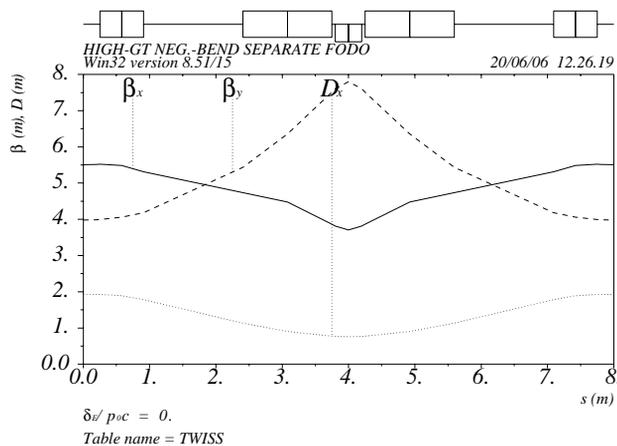
Figure 6: High- $\gamma_T$  negative-bend lattice with  $95.4^\circ$  horizontal phase advance.
