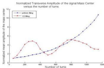
Figure 6: Vertical multibunch tracking with 2000 particles in each bunch with a small positive chromaticity.
