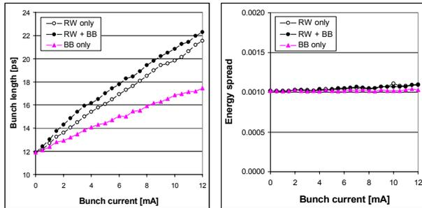
Figures 3: Bunch lengthening (left) and energy spread widening (right).
