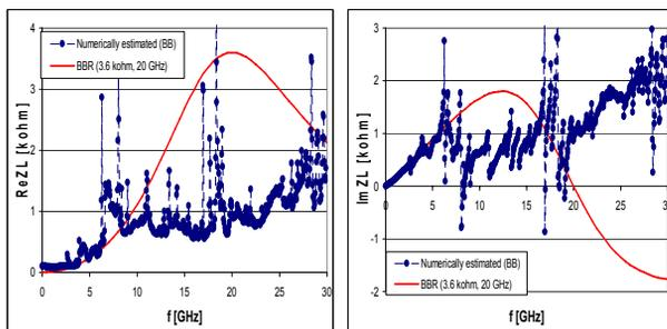
Figures 1: Numerically calculated longitudinal broadband impedance in comparison with the model employed.
