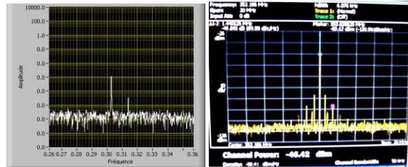
Figure 7: Observed vertical multi bunch instability. Unidentified peak in a partial fill (left) and betatron lines around the RF frequency in the uniform fill (right).
