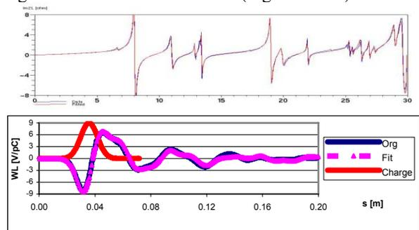
Figures 2: BPM impedance decomposition (upper) and reconstruction of a wake potential (lower).
