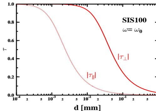
Figure 4: Comparison of transverse and longitudinal transmission coefficients for SIS 100 at revolution frequency
