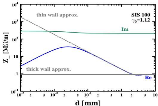
Figure 3: Transverse exact resistive wall impedances (blue, green) together with the thin wall approximation result for SIS 100
