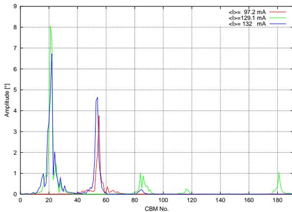
Figure 4: CBM spectra of a damped DORIS-cavity at 1.5 GeV and mean currents of 97 (red), 129 (green) and 132 mA (blue), also with this resonator CBM 21-22 and 53-55 is appearing.
