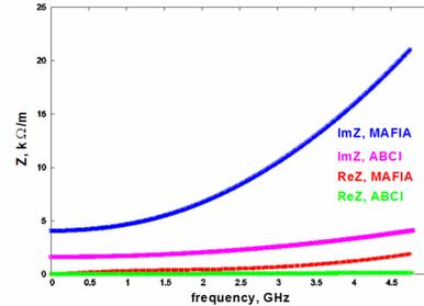
Figure 3: The PANDA insertion transverse impedance.
