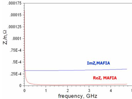
Figure 4: Longitudinal impedance of T-insertion (MAFIA).
