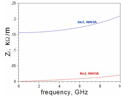
Figure 5: Transverse impedance of T-insertion (MAFIA).
