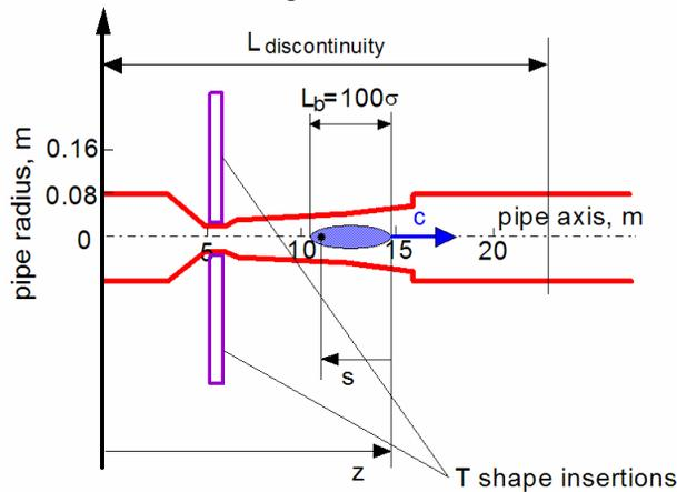
Figure 1: The longitudinal cross-section of PANDA.
