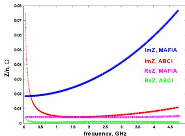
Figure 2: The PANDA insertion longitudinal impedance.
