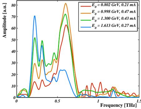
Figure 3: The spectrum in the far infrared (FIR) for different electron beam energies. The shift from higher to lower frequencies with increasing beam energy is clearly visible and denotes the increase in natural bunch length with beam energy.
