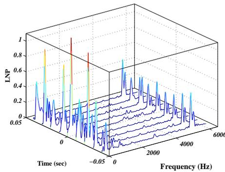
Figure 6: Lomb Normalised Periodograms of the bolometer signal during the evolution of a burst (at  $t = 0$ ). This dataset was recorded at a relatively high bunch current (0.47 mA) and at a beam energy of 1.3 GeV.
