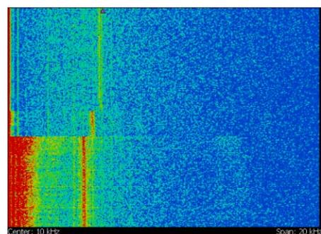
Figure 9: Spectrogram of the bolometer signal as a function of time (moves downward) during a “low  $\alpha_c$  squeeze” at a (constant) low bunch current. The steps in synchrotron frequency are clearly visible.
