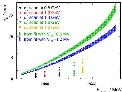
Figure 2: RMS Bunch length derived from measurements of  $f_s$  (see Fig. 1) as a function of beam energy. The hatched regions are error bands obtained by a full error Monte Carlo. The markers represent bunch lengths derived from synchrotron frequency measurements for different beam energies.
