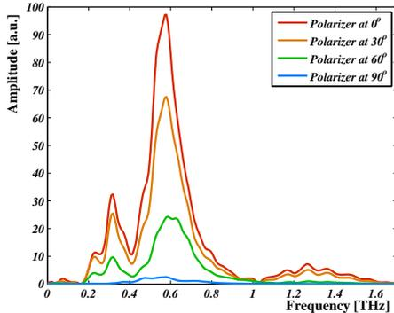
Figure 4: The FIR spectrum measured at a beam energy of 1.3 GeV ( $V_{RF} = 1.2$  MV,  $f_s = 7.1$  kHz) for different orientations of the polarising grid. The  $0^\circ$  position corresponds to a horizontal, the  $90^\circ$  to a vertical orientation.
