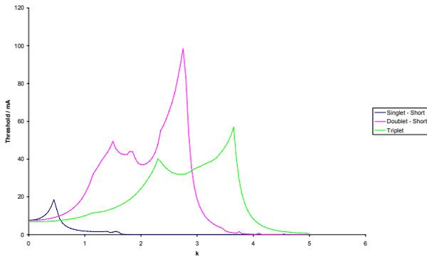
Figure 7: Threshold for changing k value with gap between modules decreasing.
