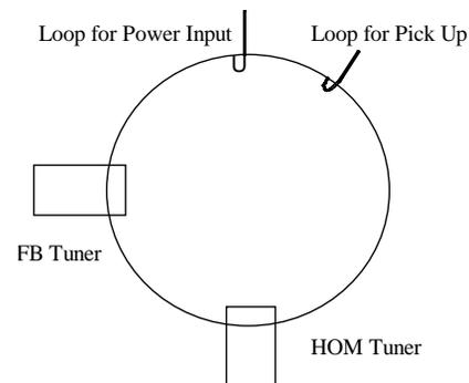
Figure 1: Cross section of the RF cavity.
