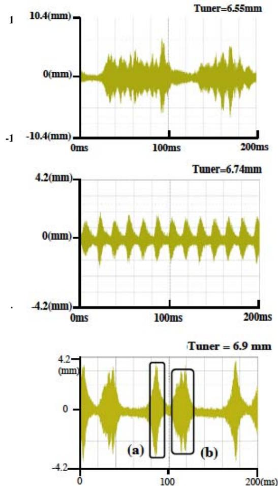
Figure 2: Outputs of the Bergoz circuit. These shows typical oscillation pattern of bunch centres.
