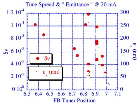
Figure 4: Estimated tune spread and emittance for Landau damping. Closed circle: tune spread, open: emittance.
