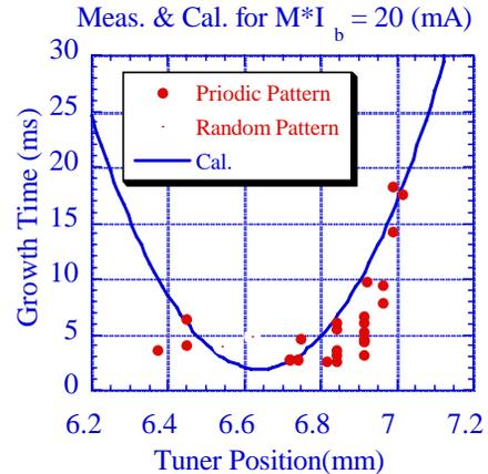
Figure 3: True growth time. Circles; measured, line ; calculation ( $l = 0$  mode).
