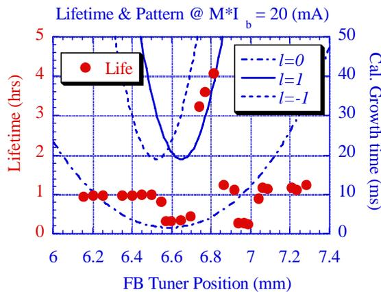
Figure 5: Lifetime and  $l = \pm 1$  mode. Beam size was large for long lifetime. Circles: lifetime, lines: growth time.
