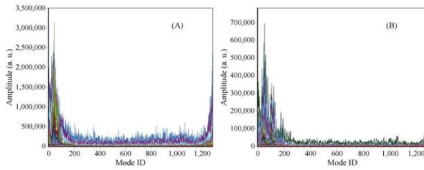
Figure 2: Observed unstable modes with 45 Gauss solenoid field for the horizontal plane (a) and the vertical plane (b)
