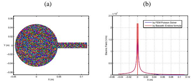
Figure 1: Triangular mesh based on KEKB antechamber geometry (a) and comparison of beam field calculation by different method (b)
