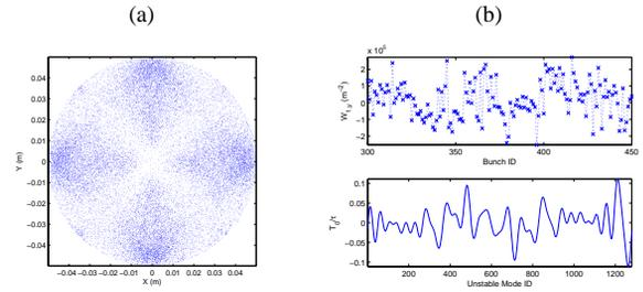
Figure 6: (a) Electron cloud distribution in the transverse x-y plane within Quadrupole magnet. (b) Wake field and growth rate of coupled-bunch instability. Initial displacement in  $+y$  direction is 5mm.
