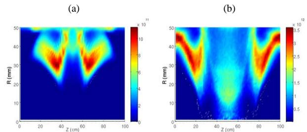
Figure 4: Electron cloud distribution in 45 Gauss EP configured solenoid field, (a) for small gap case and (b) for large gap case.
