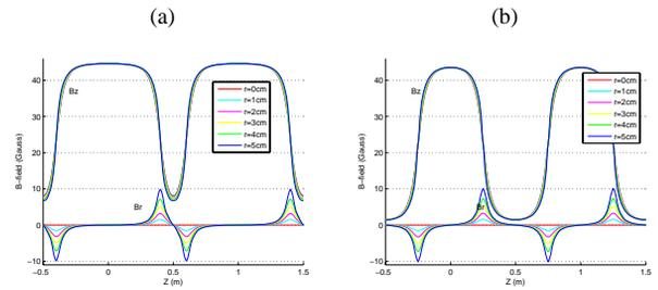
Figure 3: Realistic solenoid field within 2 equal polarity configured solenoids of  $B_0 = 45$  Gauss, 20cm gap is assumed in (a) and 50cm in (b).
