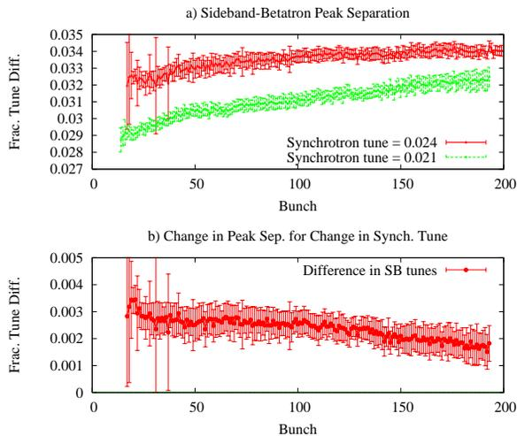
Figure 4: Effect of changing synchrotron tune (RF voltage) on sideband-betatron peak separation along train.
