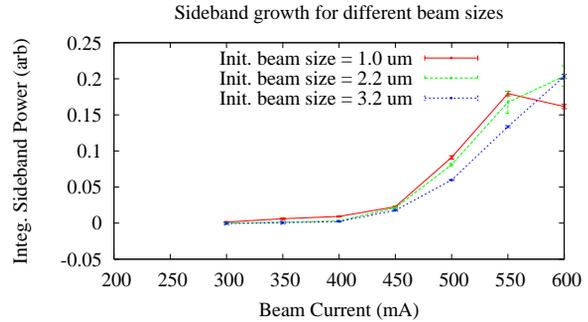
Figure 3: Effect of changing initial beam size on integrated sideband peak power along train.
