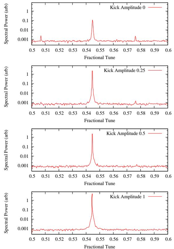
Figure 5: Effect of applying a continuous excitation at the betatron frequency on non-colliding bunch spectrum. Kick amplitude increases going from top to bottom. The vertical betatron peak is seen near 0.544 and the sideband peak near 0.577. The peak near 0.507 in the top plot is the horizontal betatron tune.
