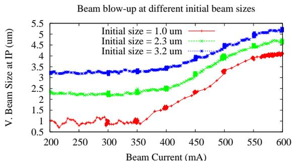
Figure 2: Beam blow-up as a function of beam current for initial beam sizes of 1, 2.3 and  $3.2 \mu\text{m}$ .
