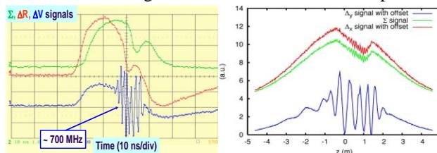
Figure 6: Measured (left) and simulated with the HEADTAIL code [9] (right) fast vertical instability in the PS near transition [10]. For the simulations a broad-band impedance model ( $R_y = 3$  M $\Omega$ /m,  $f_r = 1$  GHz and  $Q = 1$ ) was used. The hole in the longitudinal and horizontal signals reveals that some particles are lost.
