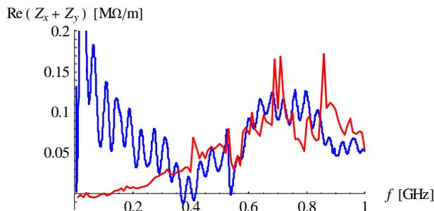
Figure 5: Comparison between the measured horizontal plus vertical driving real impedances using the single-wire (in red) and two-wire (in blue) methods.
