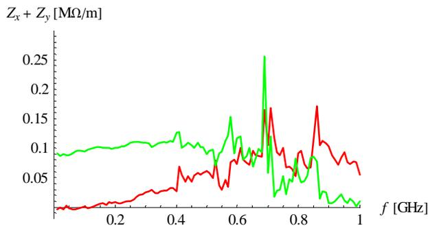
Figure 4: Measured horizontal plus vertical driving impedances. The real part is in red, whereas the imaginary part is in green.
