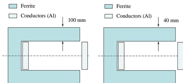
Figure 1: Cross section of the extraction kickers to be installed (left) in SS13 and SS21, and (right) in SS4.
