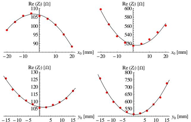
Figure 3: Measured real part of the longitudinal impedance (red dots) vs. (upper/lower) horizontal/vertical offset at 200 MHz (left) and 1 GHz (right). The full black line is the parabolic fit used to deduce the transverse impedance.
