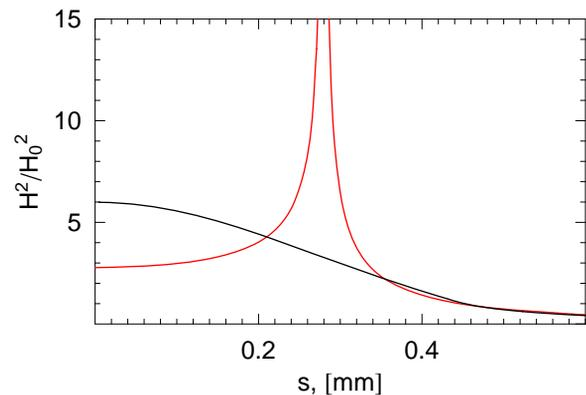
Figure 3: Normalized  $H^2$  as function of distance along the metallic surface  $s$ , for the the vacuum chamber with flat fin tips (red color) and for rounded fin tips (black curve). The point  $s = 0$  is at the bottom of the fin (the tip) in the midplane.
