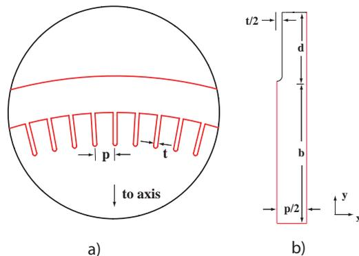
Figure 1: a)—detail of the grooved vacuum chamber wall; dimensions shown are period  $p$  and fin thickness  $t$ ; b)—geometry for the problem that is actually solved (for the case of rounded fin tips). The  $z$  axis points out of the page.
