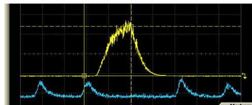
Figure 3: Beam induced signal on kicker cavity (blue). Signal induced on the cavity from cooling system (yellow). Beam induced signal is amplified by 30 dB.
