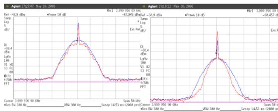
Figure 6: Schottky spectra at 4 GHz before and after cooling. Left: blue is reference spectrum before, red is signal-suppressed spectrum during cooling. Right: blue is reference, red is narrowed spectrum after cooling (system off).
