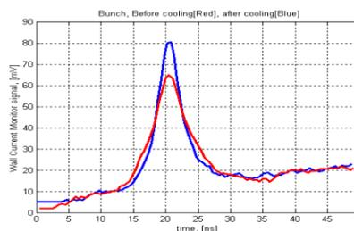
Figure 7: Test bunch, before (red) and after (blue) cooling.
