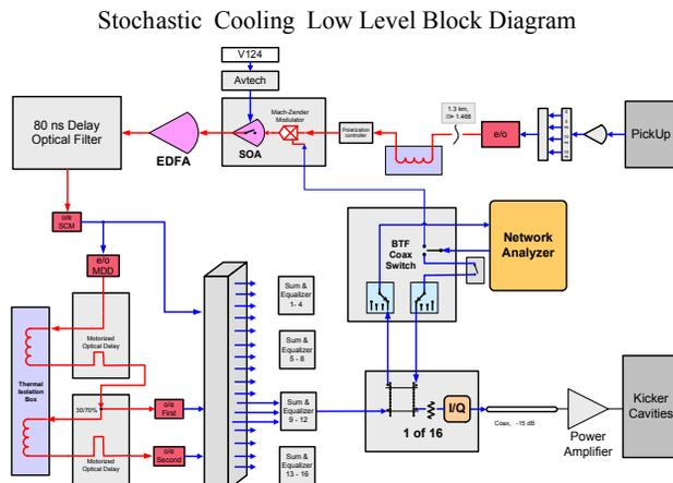
Figure 2: Block diagram of the low level electronics. Red indicates fiber optic, blue is coax. EDFA=erbium doped fiber amplifier, SOA=semiconductor optical amplifier.
