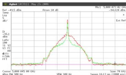
Figure 5: Signal suppression of the Schottky spectrum when the cooling loop is phased correctly. Red is open loop, green is closed.
