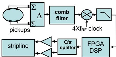
Figure 4: Layout of a transverse feedback system.
