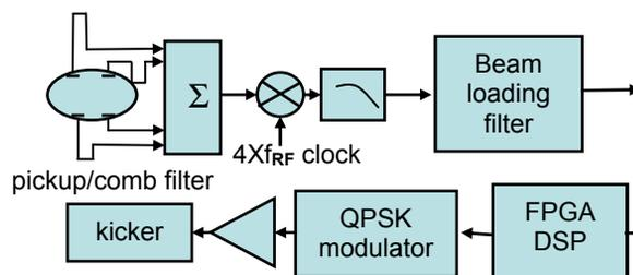
Figure 1: Layout of the ESRF longitudinal feedback.
