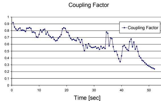
Figure 5: Change of the coupling factor while minimizing the crossplane coupling.
