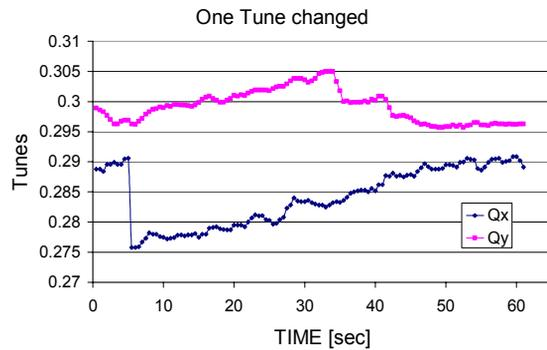
Figure 1: Reaction of the algorithm to the change of one tune.
