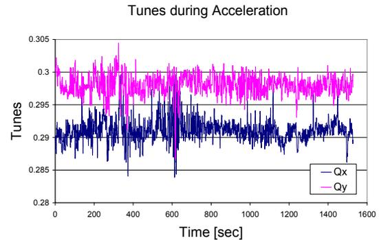
Figure 3: The tunes during acceleration.
