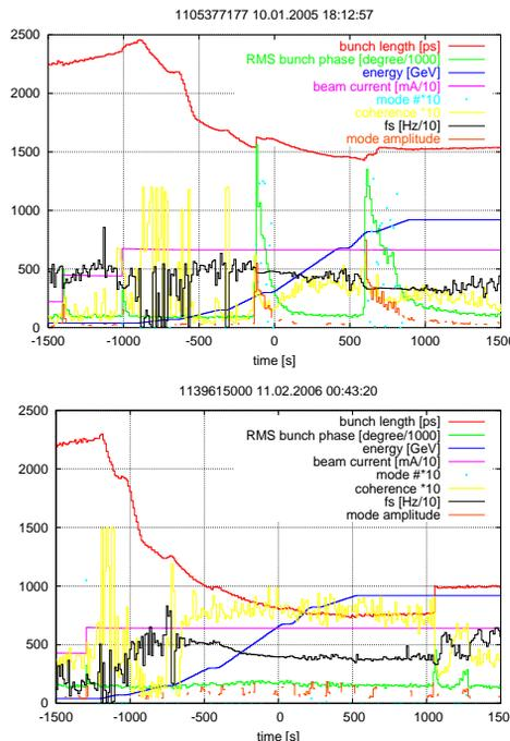
Figure 5: A typical energy ramp at HERA-p. The graph shows energy, current, mean bunch length, RMS bunch phases, measured  $f_s$  and other data derived from the FLD. The data was taken with 70 mA filled in 150 bunches. Top: Without longitudinal feedback. Bottom: With the longitudinal feedback switched on. (Here bunch length values for  $E > 300$  GeV have to be multiplied by a factor 1.45 due to calibration mismatch.)
