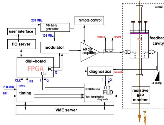
Figure 2: Overview of all components of the longitudinal feedback.
