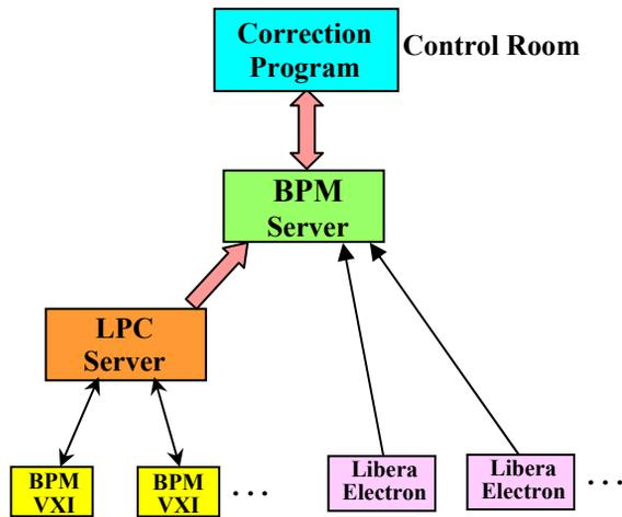
Figure 1: Block diagram of the closed orbit acquisition system that allows for a transparent operation of control room programs in the presence of old and new BPM detectors.
