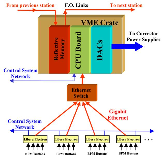
Figure 2: Layout of one of the twelve stations of the fast global orbit feedback.
