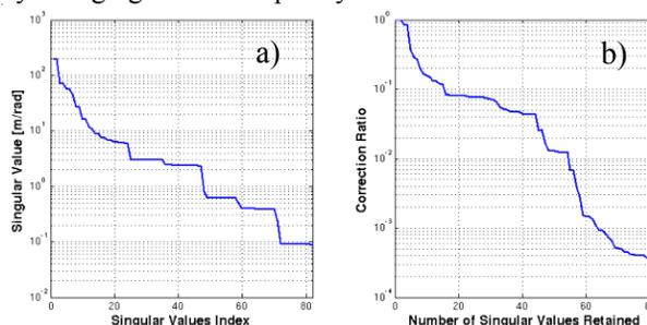
Figure 3: a) Singular values of the response matrix in descending order. b) Ratio between the *rms* of the residual and the original orbit distortion as a function of the number of singular values retained.
