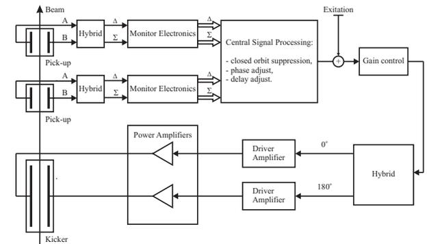
Figure 3: Layout of the transverse feedback system at the SIS100 synchrotron.
