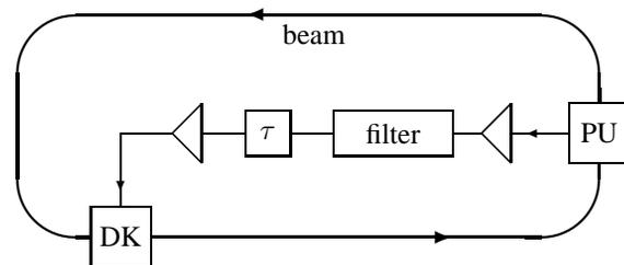
Figure 1: Layout of a transverse feedback system.
