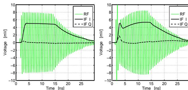
Figure 6: Simulated RF and IF signals of the  $\Delta$  channel for a beam offset of 10  $\mu\text{m}$ . Left: Ideal case without mismatches. Right: Non-ideal case with mismatches.
