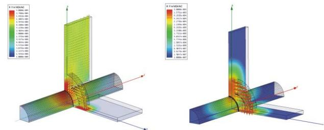
Figure 4: Left: magnetic coupling of the position sensitive  $\text{TM}_{11}$  dipole mode for the European X-FEL cavity BPM. Right: suppressed coupling of charge sensitive  $\text{TM}_{01}$  monopole mode.
