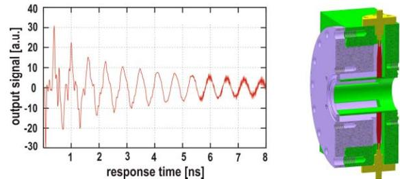
Figure 3: Left: time domain response function of the resonant stripline for the FLASH facility. Right: 3D mechanical drawing of the BPM pick-up.
