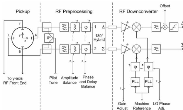
Figure 5: Proposed BPM RF front end (x-axis only).
