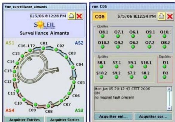
Figure 3: GlobalSCREEN application for surveying all the SOLEIL magnet defaults (water and temperature trips).
