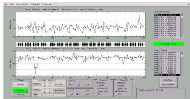
Figure 1: Plotfamily GUI used for displaying the horizontal and vertical storage ring orbit.
