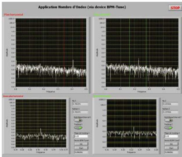
Figure 4: Tune measurement application: horizontal tune (leftside) and vertical tune (rightside) detection.
