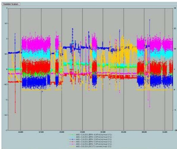
Figure 5: MAMBO application used for extraction BPM and current data over a given time span.
