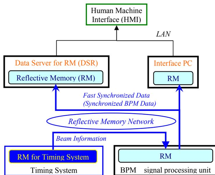
Figure 2: BPM data collection system configure
