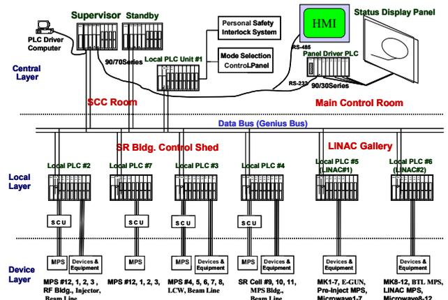
Figure 1: Configuration of MIS.
