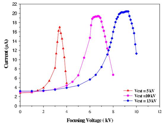
Figure 4: The helium beam currents at extracting voltage.
