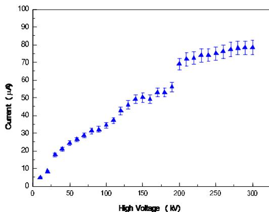
Figure 3: The beam currents at different high voltages.
