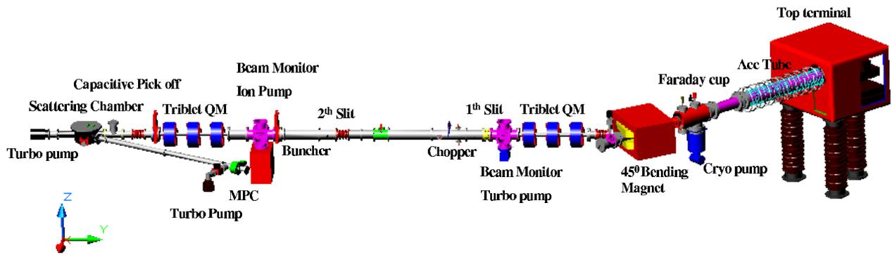
Figure 1: The He<sup>+</sup>-pulsed-beam 300-kV accelerator.
