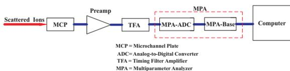
Figure 6: Electronic diagram of the backscattered-He-ions measurement.
