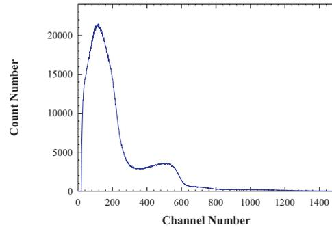
Figure 7: The spectrum of backscattered He-ions from the Si-sample with the 280-keV incident beam.
