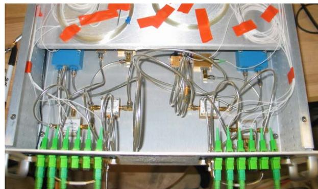
Figure 7: The comb filter chassis. Two separate filters are included, with the option on each filter to have one or two turns of delay.
