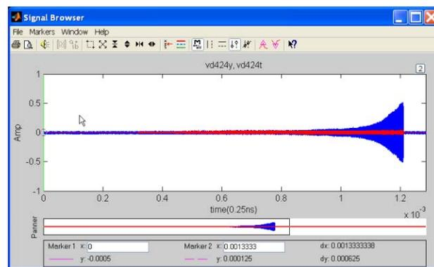
Figure 10: Sample measurement result of BPM signal. Red trace is with feedback on, blue trace is with feedback off.
