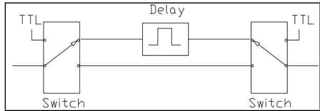
Figure 5: Schematic of binary delay line. The user can select whether to add a delay by giving a high signal to the switches, or remove a delay by giving a low signal to the switches.
