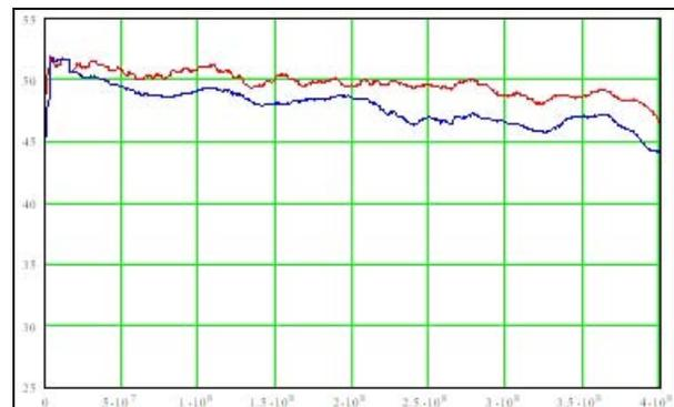
Figure 3: Gain of the power amplifiers. Notice that the gain is constant when the phase starts to drop. This is the reason for the low pass filter.
