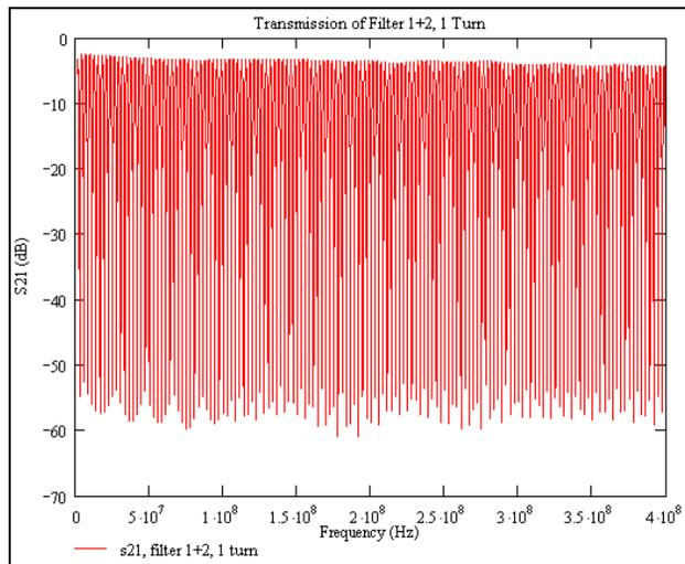
Figure 8: Measurement of notch depths for two notch filters, ganged one after the other, each having a single turn of delay.
