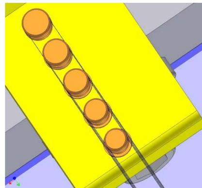
Figure 2: Turns assembly to reduce imperfections in the coil extent
