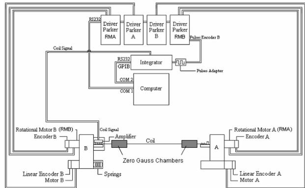
Figure 1: Schematic drawing of rotating coil system
