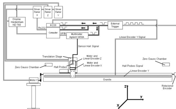
Figure 3: Set of equipment used for 3-Hall-probe scans
