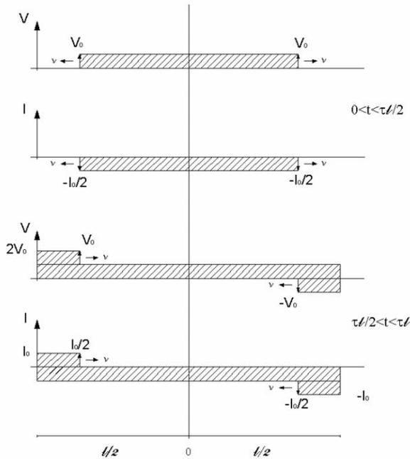
Figure 2: Diagram of the voltage and current along the storage lines.
