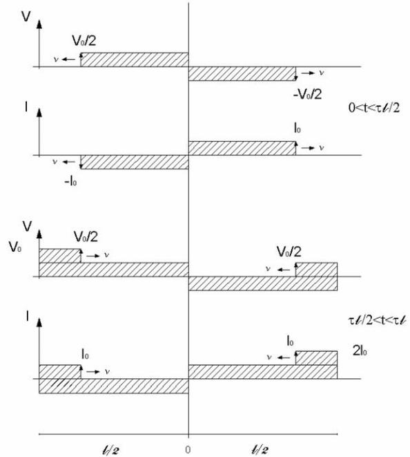
Figure 4: Diagram of the voltage and current along the storage lines.
