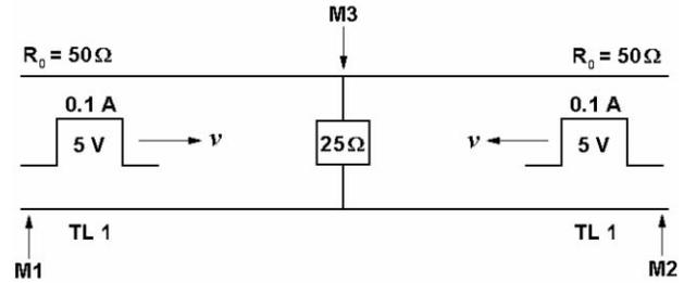
Figure 7: Experimental circuit utilised the current signal.
