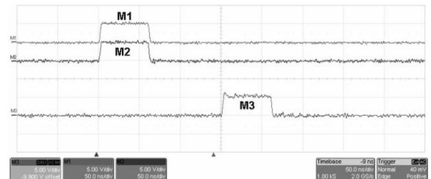
Figure 8: Experimental results. M1 and M2: input pulses. M3: Pulse measured on  $R_L$  (12.5 Ω) 0.2 A.
