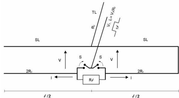
Figure 1: Schematic sketch of the VPA. S: fast switches,  $R_L$ : load resistor.
