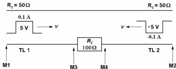
Figure 5: Experimental circuit utilised to double the voltage signal.
