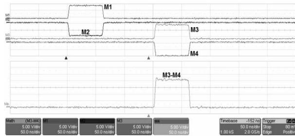
Figure 6: Experimental results. M1 and M2: input pulses. M3 and M4: Pulse measured on  $R_L$ . M3-M4: output voltage signal.
