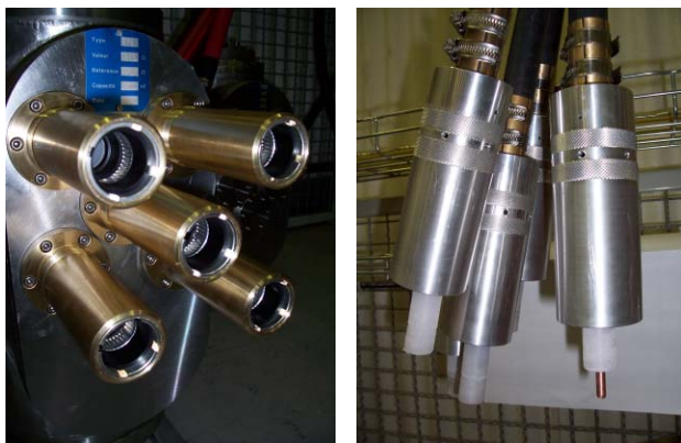
Fig. 2. Left: Connector sockets with multi-contact system; Right: RG220 high voltage cable with connectors.
