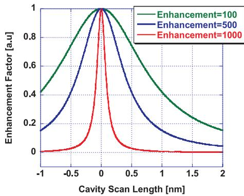
Figure 4: Resonant peak of each enhancement factors
