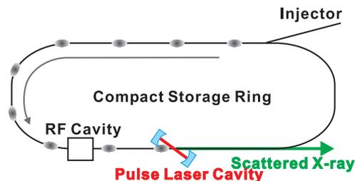
Figure 1: Schematic diagram of compact x-ray source
