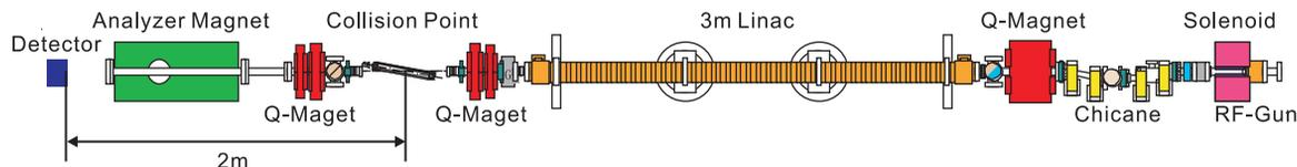
Figure 2: LUCX 50MeV beam line layout
