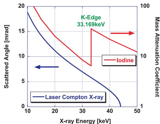
Figure 3: Laser undulator x-ray energy at LUCX
