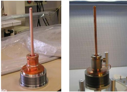
Figure 3: Prototype with disc window (left) and cylindrical window (right).
