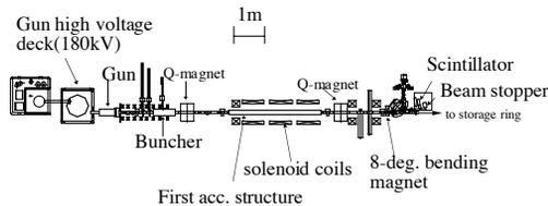
Fig.2: Dark current energy measurement system of SPring-8 injector
