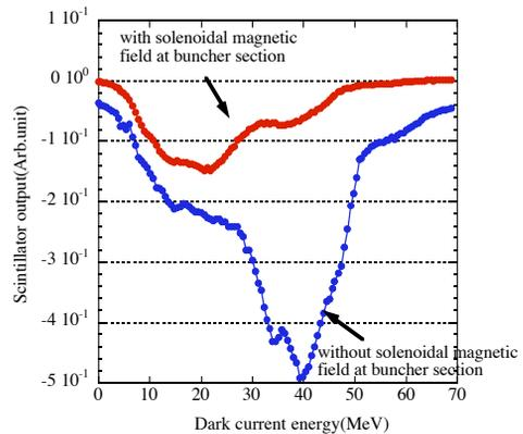
Fig. 4: The effect of the solenoidal magnetic fields on the dark currents at the injector section
