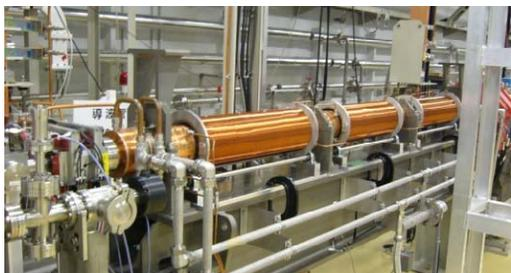
Fig. 5: solenoid coils covering the first accelerating structure.
