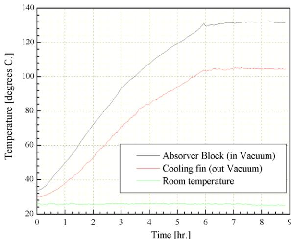
Figure 3. Cooling test at 400 Watt heating
