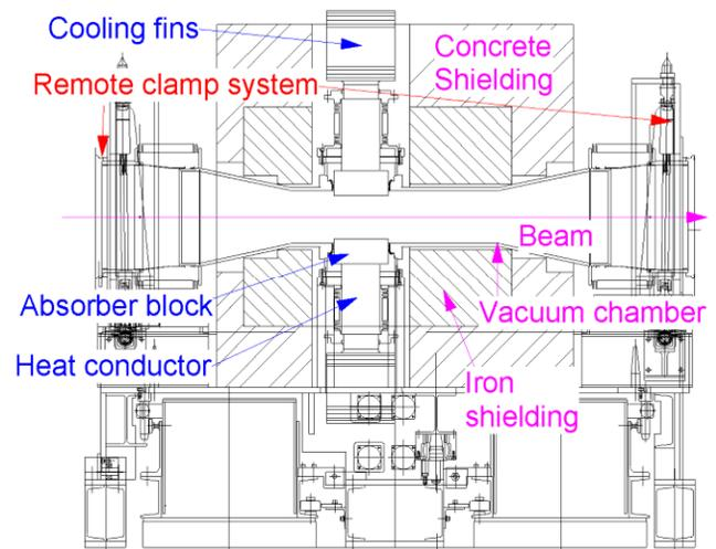
Figure 1. Schematic of J-PARC RCS collimator
