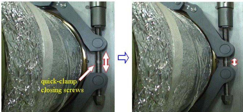
Figure 7. Close the quick-coupling clamp
