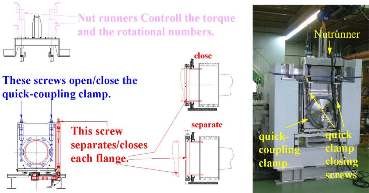
Figure 5. Schematic of the remote clamp system (left) and the nut runner setting (right)
