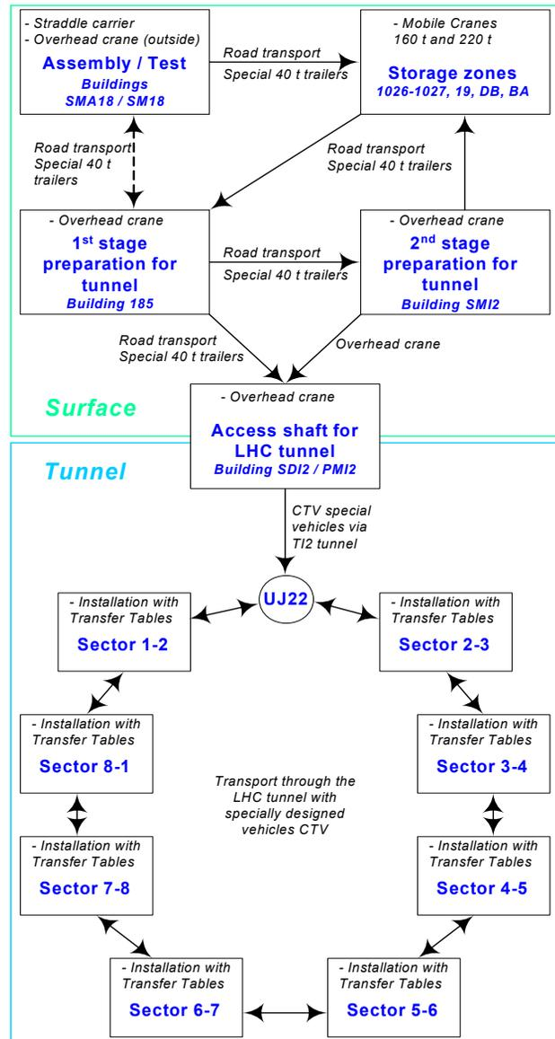
Figure 1: Cryo-dipole handling and transport sequence from surface assembly building to the final position in the LHC tunnel.
