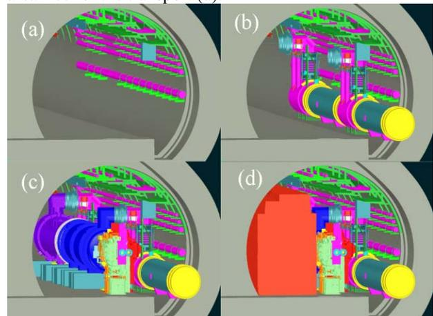
Figure 2: Phases of the LHC Machine Installation.
