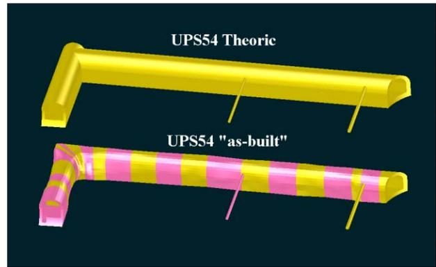
Figure 8: Tunnel as-built model from scanned points.
