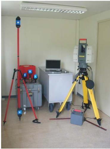
Figure 3: Leica laser HDS3000 and its accessories.
