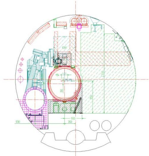
Figure 1: Typical Section of the LHC Tunnel.
