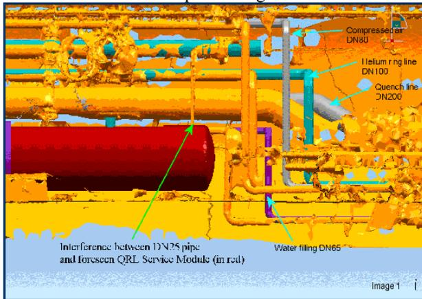
Figure 7: Interference identification.
