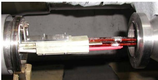
Figure 3: Insulated splice in GFRE support.
